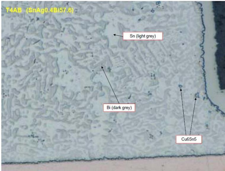
**Figure 28: Sn57.6Bi0.4Ag soldered 3216[1206] chip component cross-section.**
