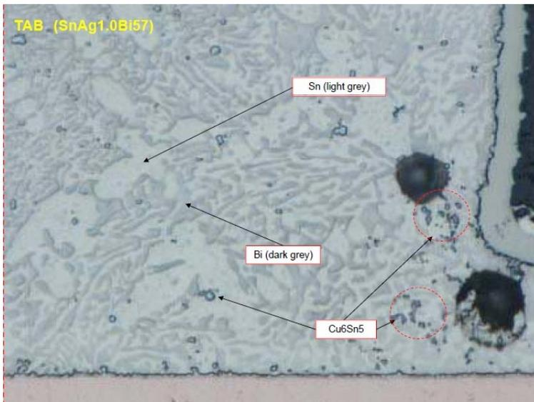
**Figure 29: Sn57Bi1Ag soldered 3216[1206] chip component cross-section.**
