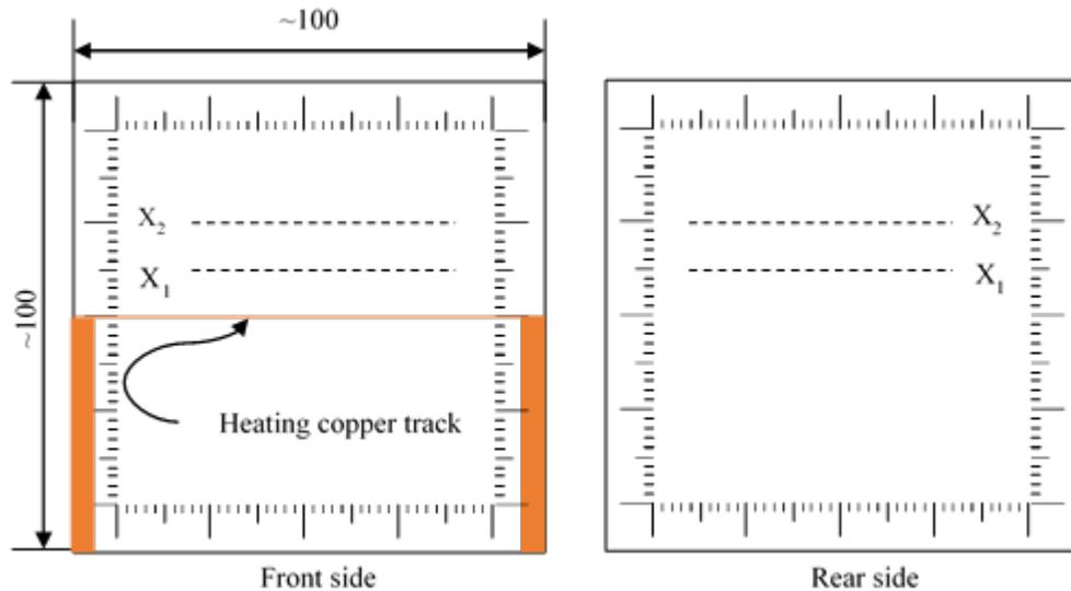
**Figure 6: Transient fin sample design**
