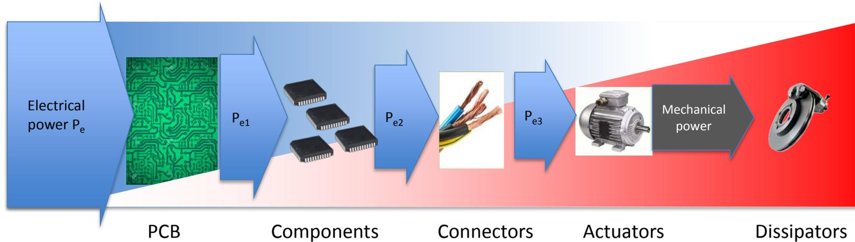
Electrical energy brought to a system is almost integrally turned into heat, *but not necessarily locally*, and that is a reason of problems for PCB designers...
