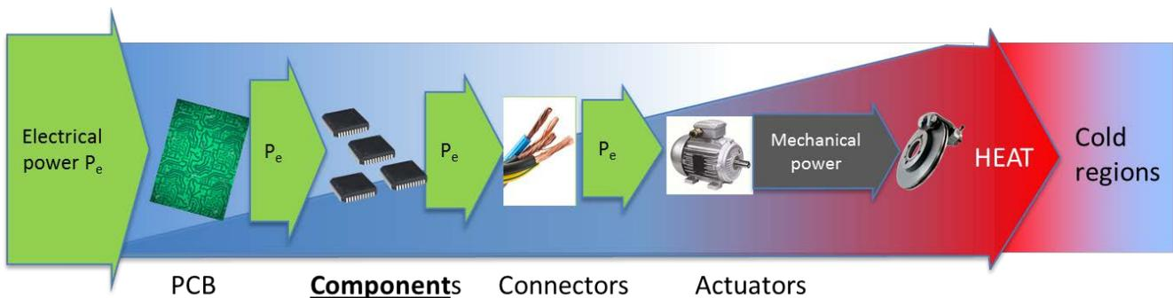
Heat is generated all along the chain. At the electronic system level, the main contributors are often components. The printed circuit board, supporting and interconnecting them, is also very helpful to avoid system excessive heating. Indeed, excessive temperatures degrade overall system performance, from speed to long term reliability. Therefore, electronic system designers take great care of operating temperatures. Equations managing thermal exchanges can be easily found in the literature.
