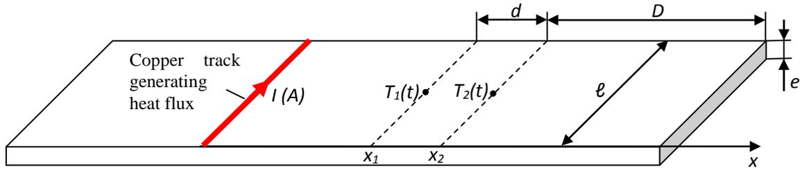
**Figure 4: Transient fin method principle**
