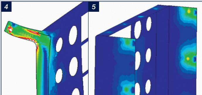
Figure 4: Stress analysis of aluminum bracket showing overstress at mounting tab.
