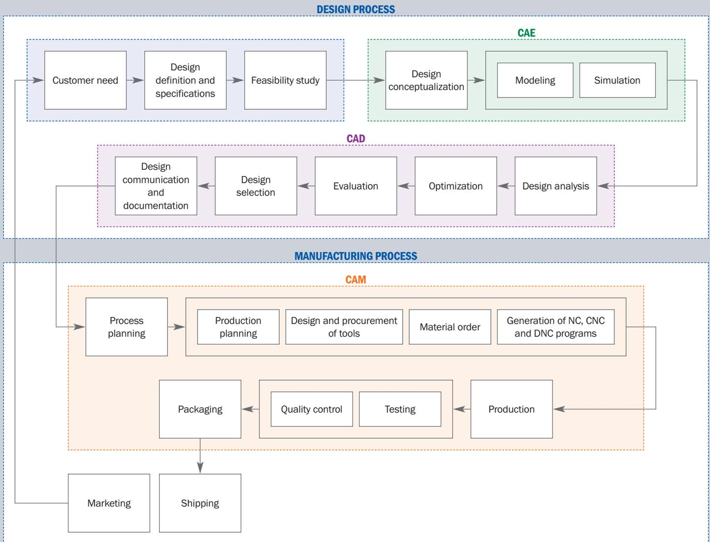
Figure 1: The product cycle from design to production.
