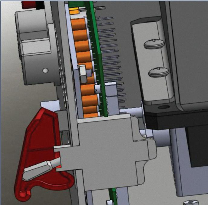
*Figure 2: CAM assembly model containing COTS and custom parts to check for interferences.*
