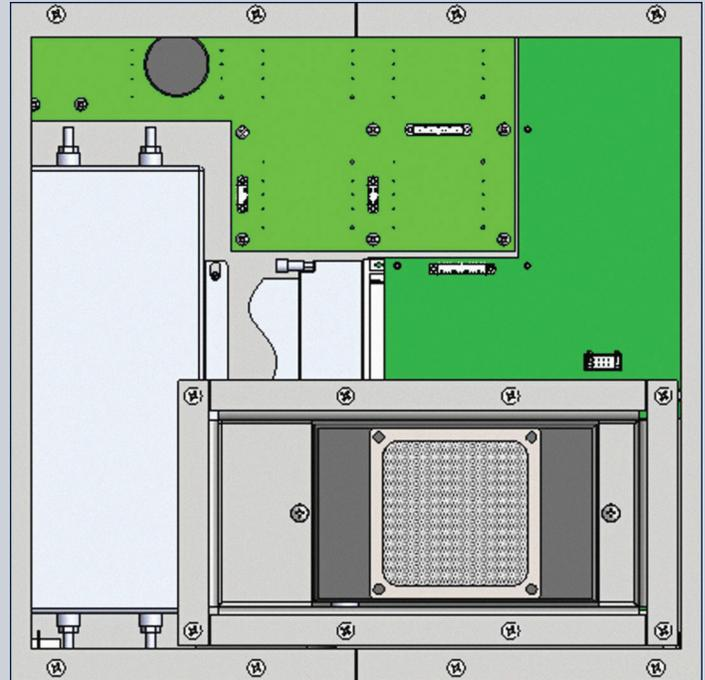
*Figure 3: Three dimensional model showing how board shape (green) was designed to fit with other COTS components (grey).*
