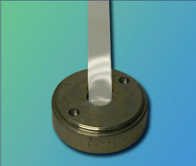
Figure 2: Fixture containing encapsulated test circuit board.
