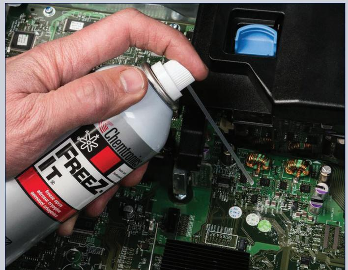
*Figure 1: Freeze spray is an essential tool, because it helps identify faulty components, solder joints, and other problems that can lead to board failure. Photo courtesy of Chemtronics.*
