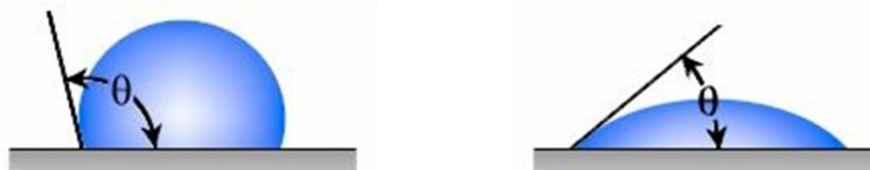
Figure 4: Explanation of Contact Angle and Hydrophobicity
