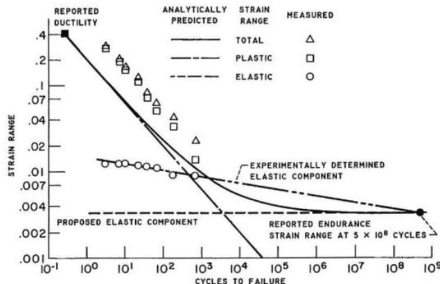
Figure 1: Fatigue curve of 24ST aluminum, showing low cycle and high cycle fatigue<sup>6</sup>
