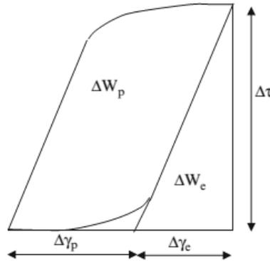
Figure 4: Representative schematic of a solder joint hysteresis loop<sup>19</sup>
