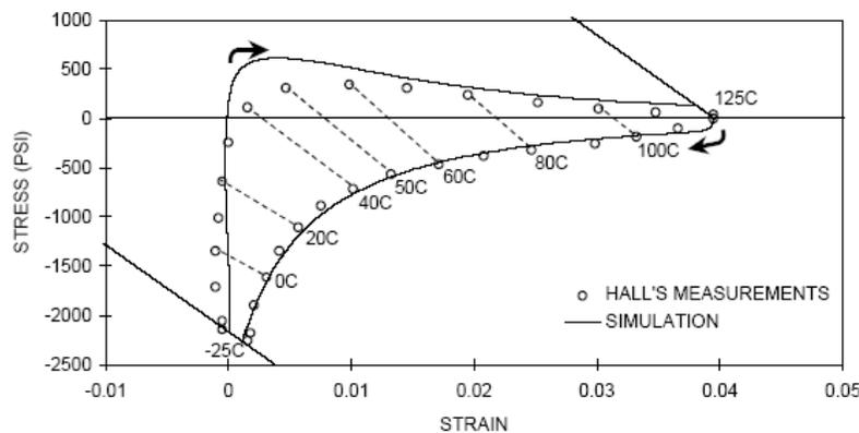
Figure 3: Hysteresis loop of a leadless ceramic chip carrier solder joint during thermal cycling between  $-25^{\circ}\text{C}$  and  $125^{\circ}\text{C}$ <sup>16</sup> (obtained through [http://www.msed.nist.gov/solder/clech/Sn-Pb\\_Creep.htm](http://www.msed.nist.gov/solder/clech/Sn-Pb_Creep.htm))
