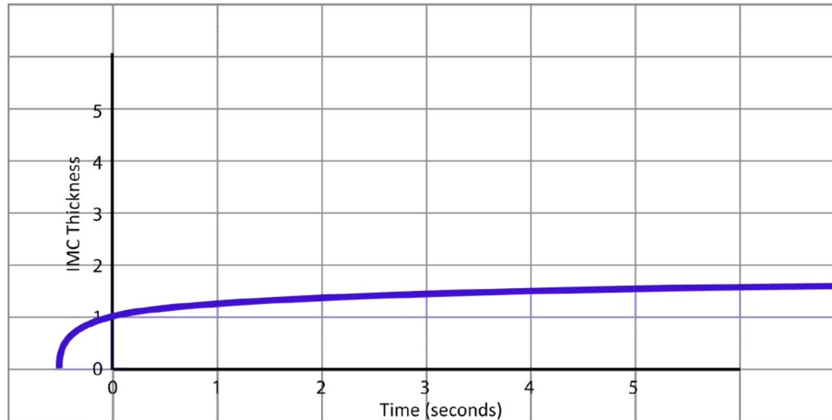
The role of intermetallic compounds (IMC) is critical to the successful formation of a solder joint. With too little IMC formation, typically  $<0.25 \mu\text{m}$ , the solder joint is cold or dry, which hinders electrical connection. Too much IMC, typically  $>4\mu\text{m}$ , solder joint embrittlement becomes a factor.
