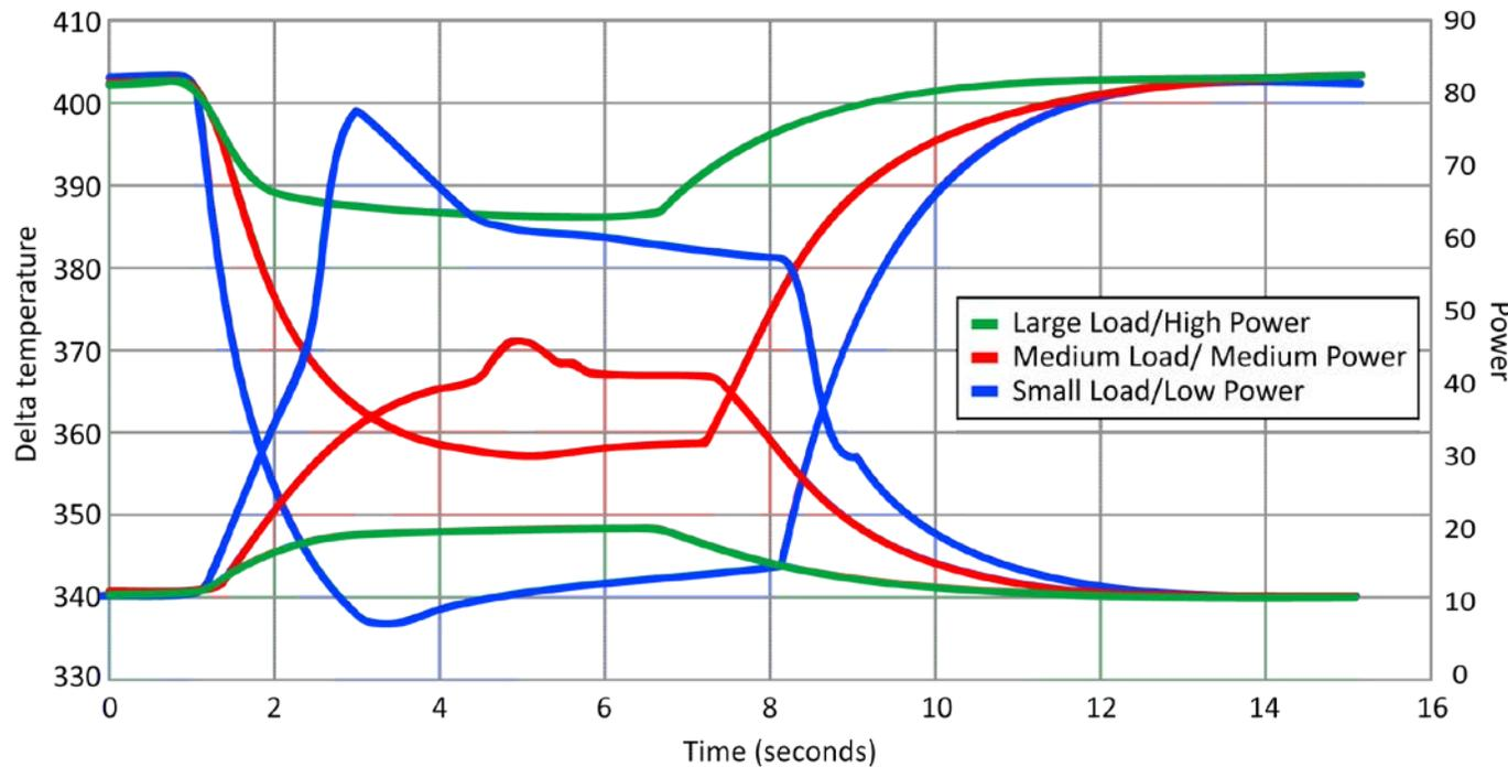
Total thermal resistance is a function of minimum thermal resistance plus maximum thermal resistance as a function of a thermal efficiency of the tip geometry over time.
