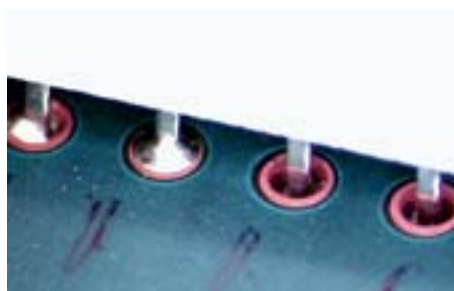
Figure 5 A: Visual inspection of specific through-hole vias
