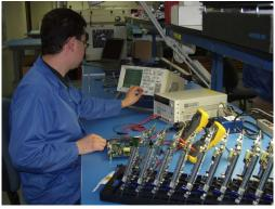
Are all ECOs documented? Is the testing procedure repeatable? A *golden* board should be made available for testing before a given batch is started. This provides the test engineer a reference point, if necessary during the test procedures. Plus, the more precise CAD tools used for DFT such as generating a netlist from a design database verses gerber generated netlist. The more accurate the testing results would be, the less time would be required to debug the board(See Fig # 4 below).
