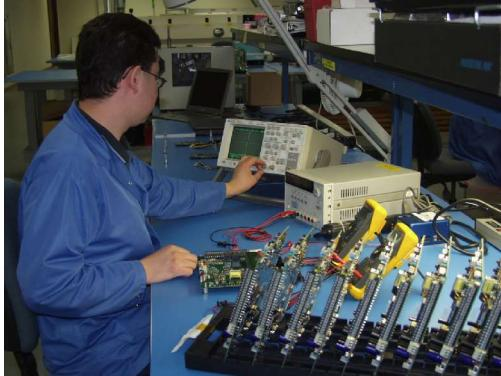
Are all ECOs documented? Is the testing procedure repeatable? A *golden* board should be made available for testing before a given batch is started. This provides the test engineer a reference point, if necessary during the test procedures. Plus, the more precise CAD tools used for DFT such as generating a netlist from a design database verses gerber generated netlist. The more accurate the testing results would be, the less time would be required to debug the board(See Fig # 4 below).
