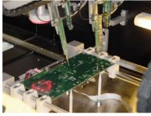
Sometimes, both the top and bottom probes may not be able to be run at the same time. Hence, it is highly recommended that all test points be laid out on the same side of the board.
