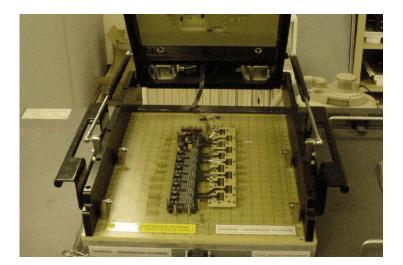
It is prudent not to make many fixture changes, even if there are changes made in the design, fixture changes should be kept to a bare minimum, to avoid extreme costs that are associated with the fixture changes. The same test fixture can be used for small changes (10% or less), but for the bigger changes, the fixture needs to be redesigned, thus costing huge sums of money.
