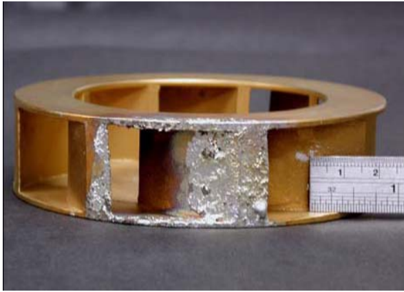
Figure 6 – TiN coated 316 stainless steel impellor
