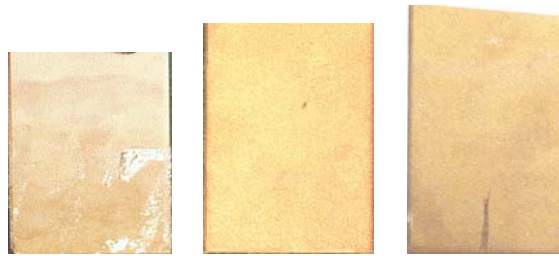
Figure 4 -Titanium Samples After Sn/Ag Exposure
