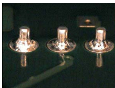
Figure 7. Various through-hole parts showing excellent wetting on top and bottom-side
