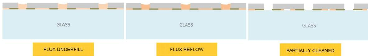
**Figure 6: Preparing the Glass Slide for Cleaning Evaluation**
