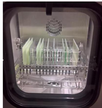
Figure 12: Batch Dishwasher Style Cleaning Machine using Linear Spray Manifolds
