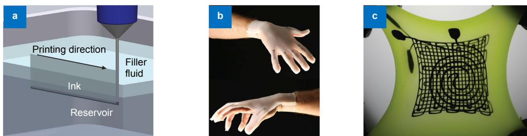
**Fig. 9 | Schematic illustration of the embedded 3D printing (e-3DP) process and printed stretchable electronics.** (a) Schematic illustration of the e-3DP process. (b) Photograph of a glove with embedded strain sensors produced by e-3DP. (c) Photograph of a three-layer strain and pressure sensor in the stretched state. Figure reproduced from ref. <sup>11</sup>, WILEY-VCH Verlag GmbH & Co. KGaA, Weinheim.
