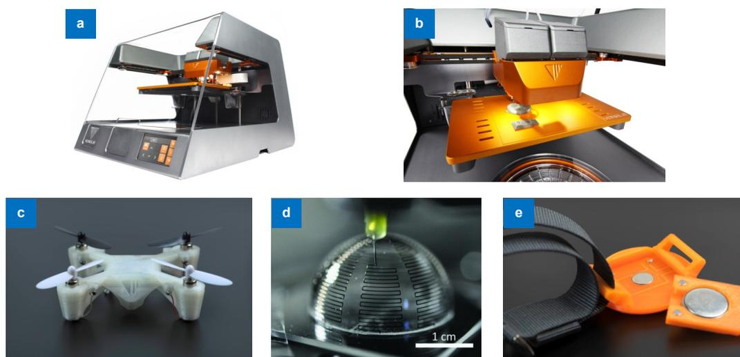
**Fig. 13 | Voxel8 and some printed products.** (a, b) Photograph of Voxel8 3D printer. (c) Printed unmanned aerial vehicle. (d) Printed antenna (dome). (e) Printed wearable device. Figure reproduced from ref. <sup>32</sup>, Voxel8.
