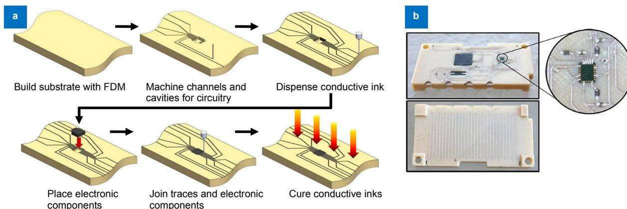
Fig. 2 | (a) Process flow of the multi<sup>3D</sup> system. (b) Fabricated parts. Figure adapted from ref. <sup>9</sup>, Springer International Publishing AG.
