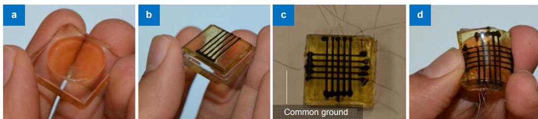
**Fig. 10 | Fabricated stretchable tactile sensor using integrated PSL and DP processes.** (a) An example (partial sphere) of 3D structure built in the PSL system. (b) Printed sensing elements using the DP process on the insulating layers built in the PSL system. (c) Final sensor with two sensing layers. (d) Deformed sensor. Figure reproduced from ref. <sup>27</sup>, Wiley-VCH Verlag GmbH & Co. KGaA, Weinheim.
