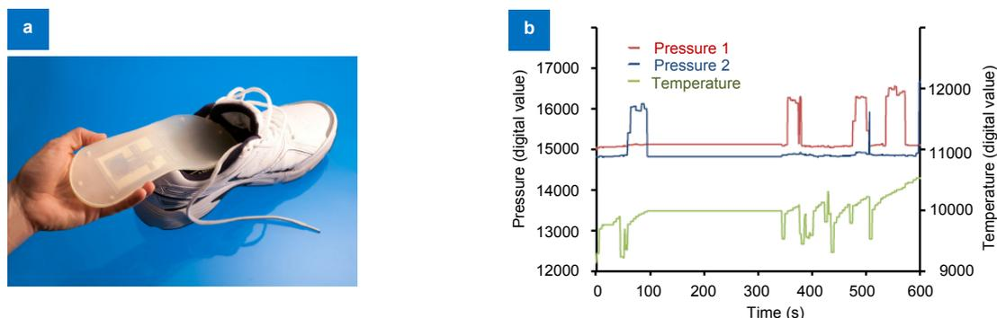
Fig. 4 | (a) Printed wireless pressure and temperature sensor within a shoe's insole. (b) Pressure and temperature data obtained through wireless communication from the printed insole<sup>22</sup>. Figure reproduced from ref. <sup>22</sup>, Society for Imaging Science and Technology.
