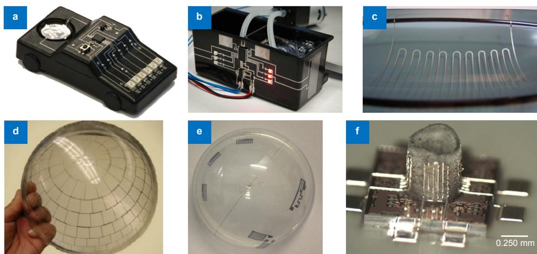
**Fig. 11 | 3D printed electronics using Aerosol Jet printing from Optomec.** (a) 3D MID demonstrator. (b) 3D MID with integrated sensor. (c) Printed conformal electronics (curve). (d) Printed conformal electronics (dome). (e) Printed conformal electronics (dome). (f) Sub-mm length scale, custom made 3D metal-dielectric. Figure reproduced from (a–c) ref. <sup>28</sup>, Neotech; (d–f) ref. <sup>29</sup>, Optomec.
