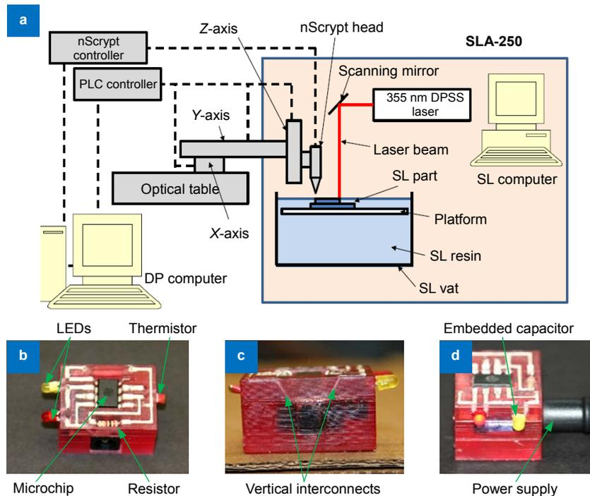
Fig. 6 | (a) Schematic of the hybrid SL/DP system. (b–d) Fabricated 3D 555 timer circuits packaged within SL substrates. Figure reproduced from: (b–d) ref. <sup>24</sup>, Emerald Publishing Limited.
