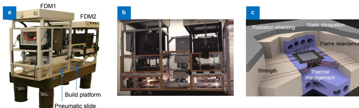
**Fig. 1** | (a, b) Photograph of the multi<sup>3D</sup> system. (c) Schematic of a fabrication example. Figure reproduced from: (a) ref. <sup>9</sup>, Springer International Publishing AG; (b) ref. <sup>14</sup>, Elsevier Ltd; (c) ref. <sup>9</sup>, Springer International Publishing AG.
