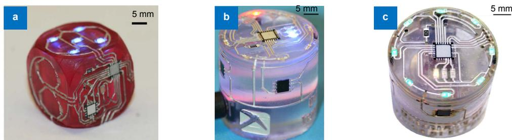
**Fig. 8 | Examples of printed 3D structural electronics.** (a) A gaming die which includes a microcontroller and accelerometer. (b, c) A magnetometer system with microprocessor and orthogonal Hall Effect sensors. Figure reproduced from ref. <sup>18</sup>, Taylor & Francis.
