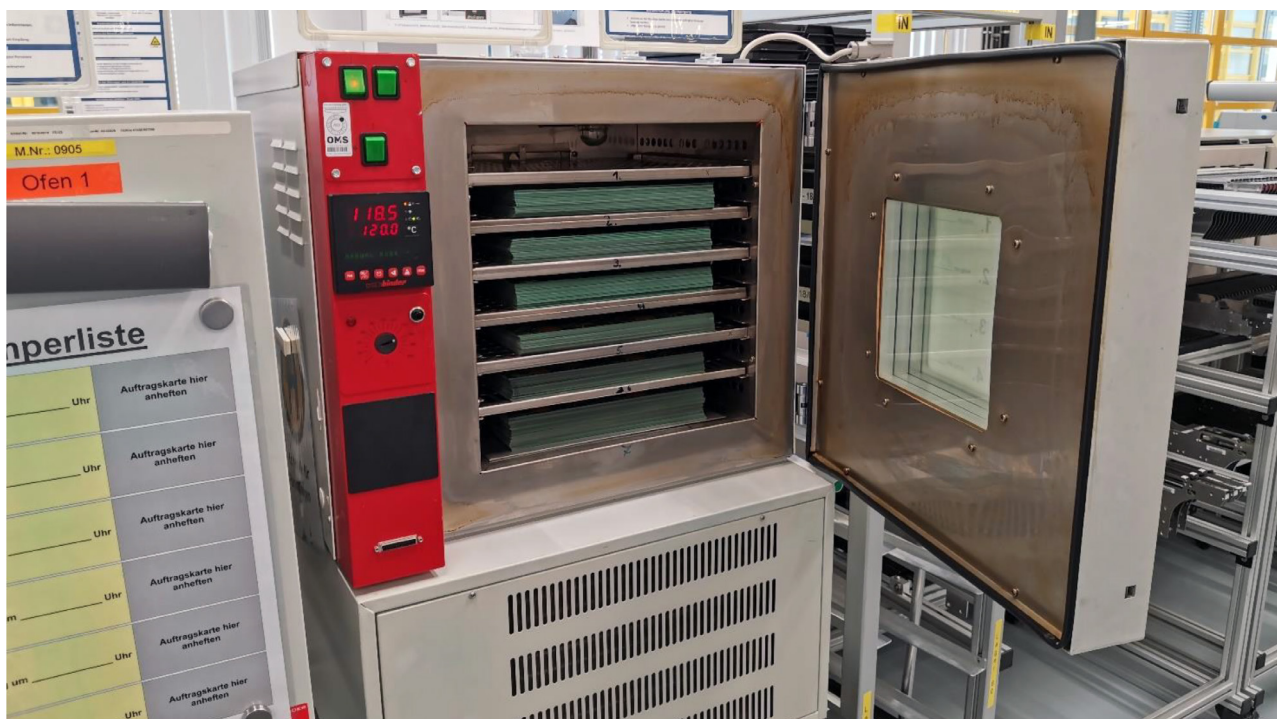
Abbildung 34: Serial process drying stage 1 in the circulating air drying cabinet at BASLER [12].
