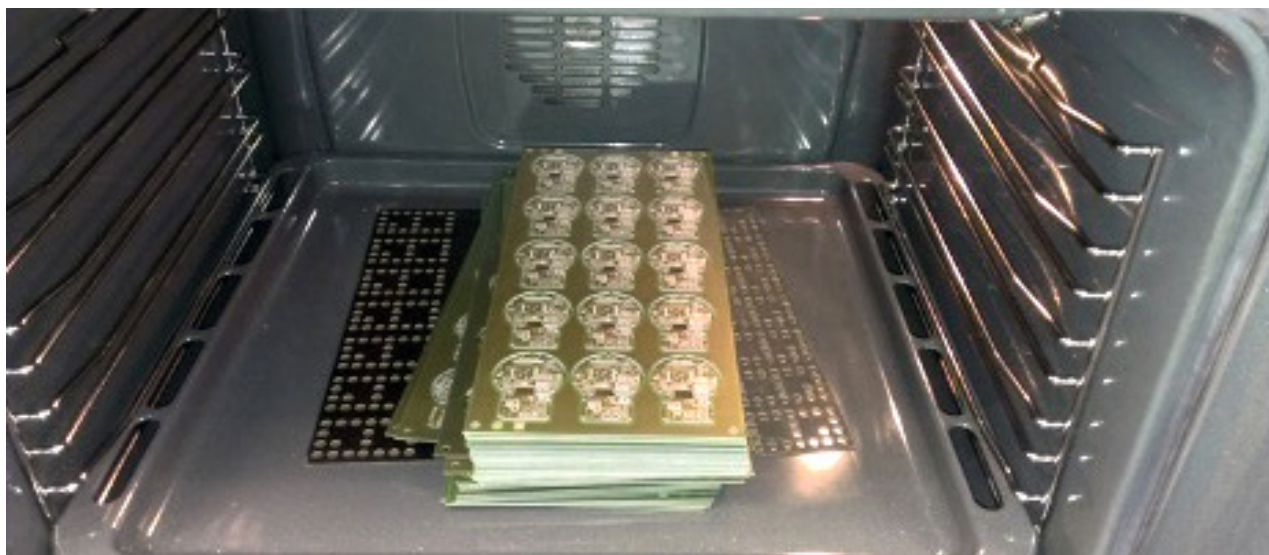
Figure 36: Two serious errors: Stack of rigid-flex PCBs clearly too thick and unsuitable oven
