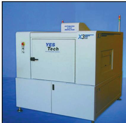
*Automated X-ray inspection system YTX-X3 can provide 3D imaging.*
