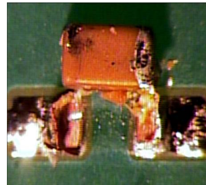
Figure 4b: Fail – Any Flux residue detected at 40X
