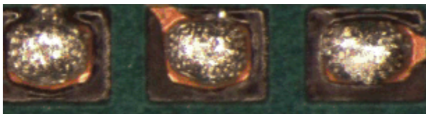
Figure 3: Partially coalesced solder on fine deposits appears as a grape-like cluster.
