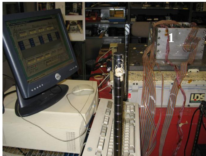
Figure 15: Resistance Monitoring System Set Up
