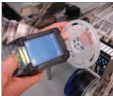
Figure 4. Reels can be scanned offline to register the relocation of the reel to the feeder trolley, or back to the storage system.
