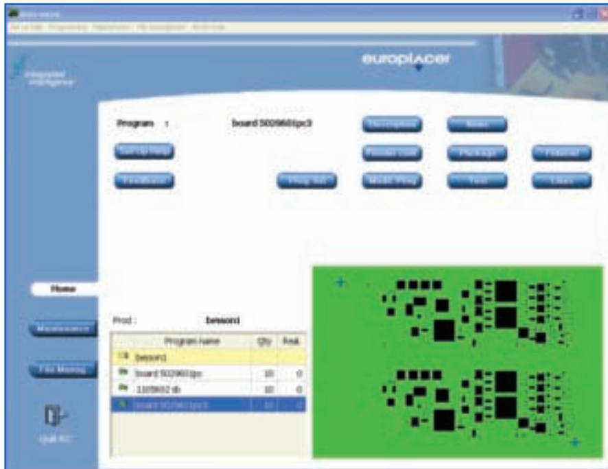
Figure 6. GUI representation of a board being setup for multi-programming.
