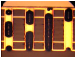
Figure 6: Cross-section of Unfilled Thermal Vias [5]
