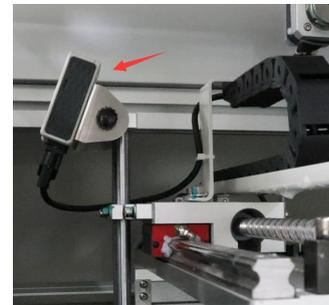
This device is used to receiving marking position data of PCB from laser marking machine and automatically scanning the position(Industry 4.0).
