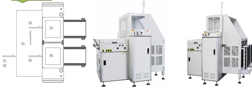
1. This device is used to receive board SMT circuit board production line operation, suitable for receive NG board and OK board after soldering.
