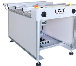
1. This equipment is usually used to transfer and cooling PCBA after reflow soldering.
