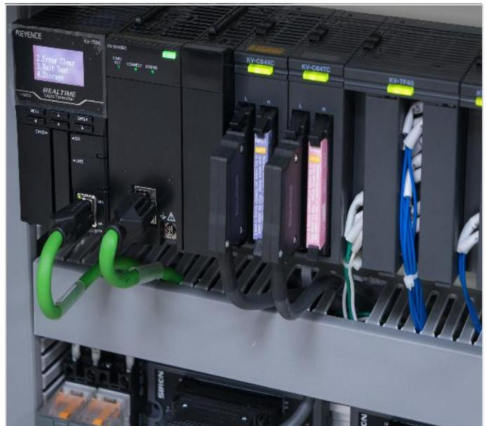
1. Keyence KV7500 PLC+Keyence module high-end bus control system, ensure the stability and extensibility of the system.
