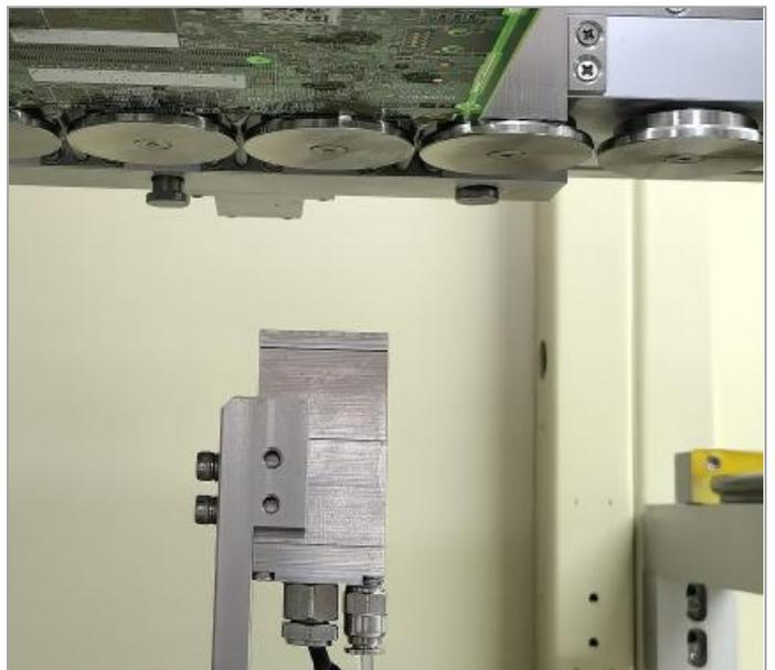
1. German high-frequency pulse injection valve to get precious fluxing result with small flux dot, flux solid content should be less than 10%. The flux nozzle jam detection function is optional.
