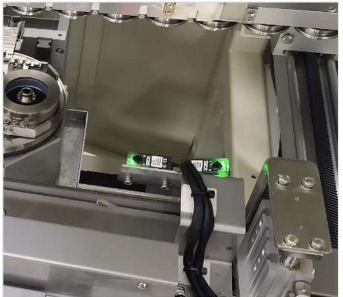
8. The transportation buffer zone is set to ensure the smooth operation of PCBA without collision.
