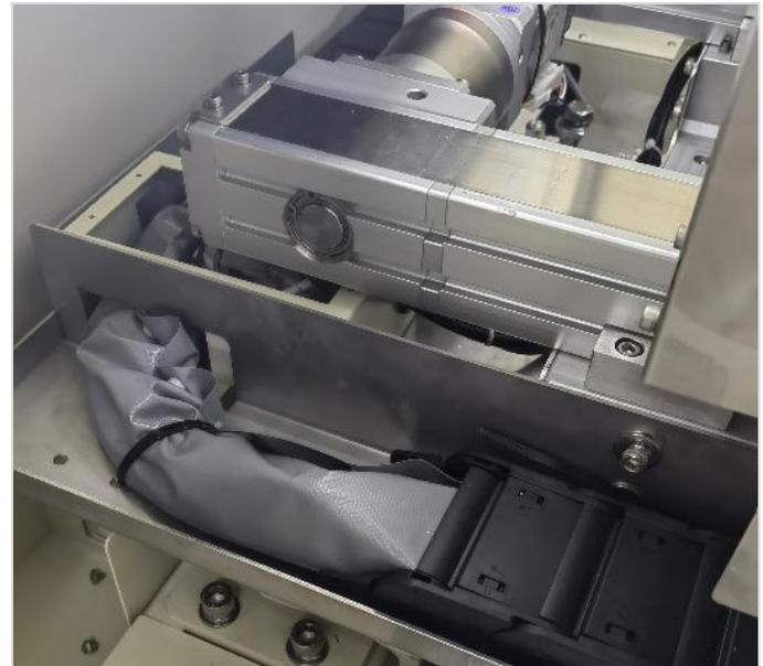
8. XYZ platform is composed of high precision lightweight sports module and high-speed servo motor.
