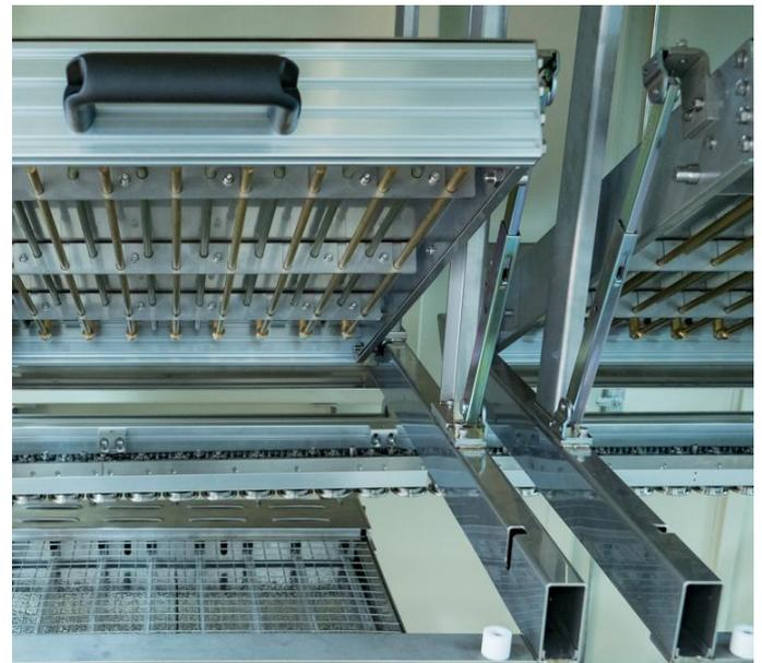
1. The machine is equipped with bottom IR preheating as standard, and the preheating area can be set; top hot air preheating, infrared heating Conduction is efficient and stable.
