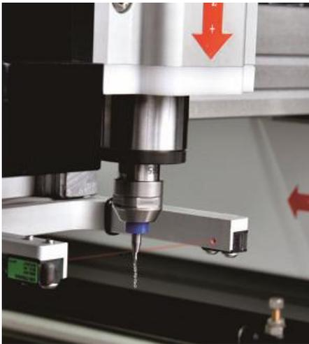
**Milling Cutter Detection**
