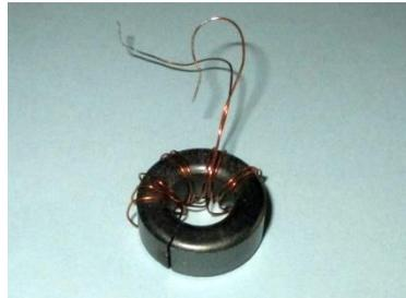
Figure 3, Example of a Gapped Toroid
