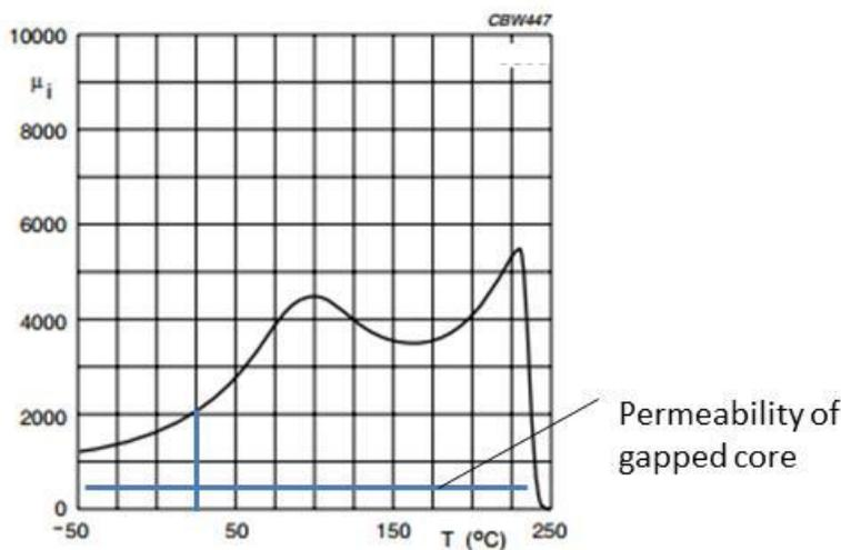
Figure 4, Ferrite permeability versus temperature (1500 permeability @ 25C)
