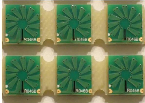
Figure 6, Laser gapped embedded inductors, 10 Winding Configuration
