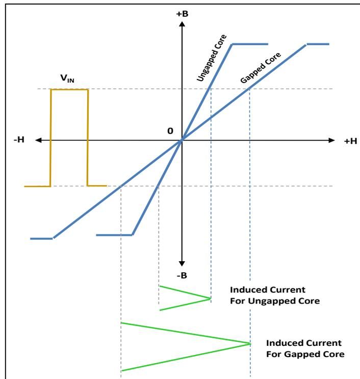
Figure 2, Typical B-H graph for an ungapped and gapped ferrite core
