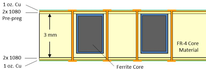
Figure 5, Test Coupon Cross Section
