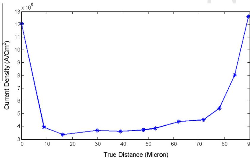
Fig. 3. Current density distribution along diagonal cross-section A-B during PDC loading history.
