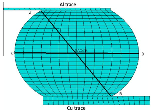
Fig. 1. Finite element mesh and electric potential gradient distribution of simulated model.
