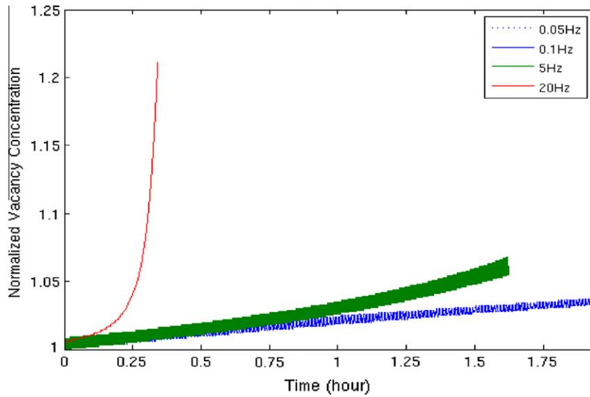
Fig. 6. Frequency dependence of vacancy concentration evolution at corner B (cathode), with maximum current density  $j_B = 2.0 \times 10^6$  A/cm<sup>2</sup> and duty factor of 0.5.
