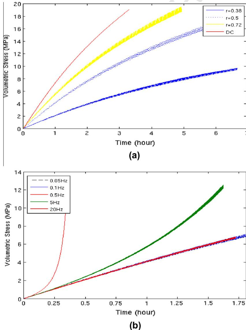
Fig. 8. Volumetric stress evolution at cathode side of the solder joint subjected to 0.05 Hz PDC with maximum current density  $j_b = 2.0 \times 10^6$  A/cm<sup>2</sup>: (a) duty factor dependence and (b) frequency dependence.
