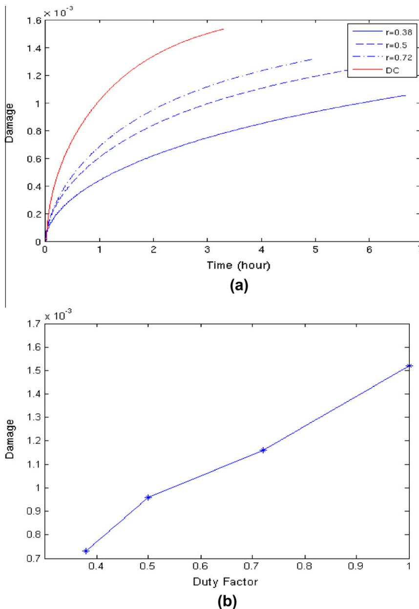
Fig. 12. Damage at cathode side of the solder joint for various duty factors with pulse frequency of 0.05 Hz: (a) damage evolution history and (b) damage vs. duty factor after 3.3 h of current loadings.
