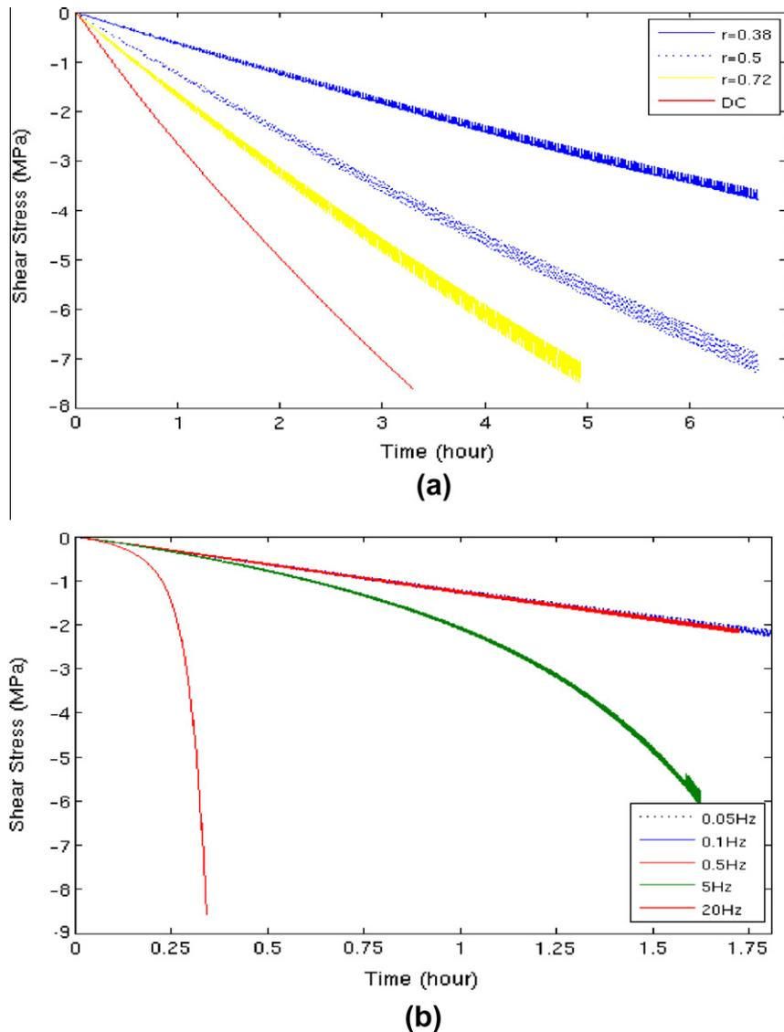
Fig. 9. Shear stress evolution at cathode side of the solder joint subjected to 0.05 Hz PDC with maximum current density  $j_B = 2.0 \times 10^6$  A/cm<sup>2</sup>: (a) duty factor dependence and (b) frequency dependence.
