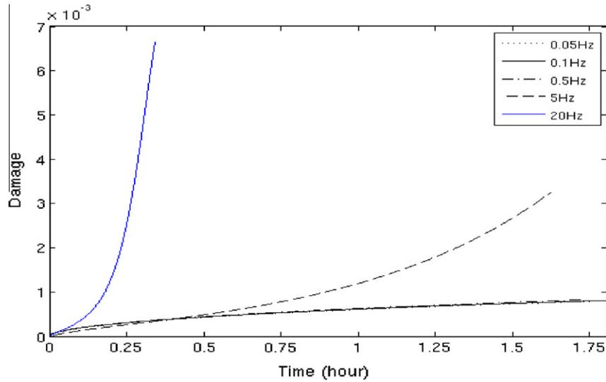
Fig. 13. Frequency dependence of damage evolution at cathode side of the solder joint subject to PDC loading with duty factor of 0.5.
