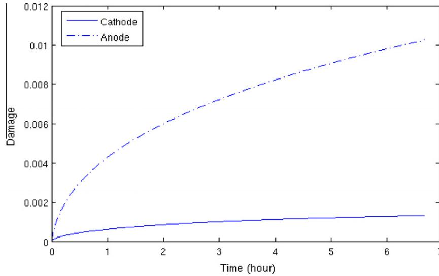
Fig. 10. Damage evolutions at cathode and anode sides of the solder joint subjected to 0.05 Hz PDC loading with duty factor of 0.5.
