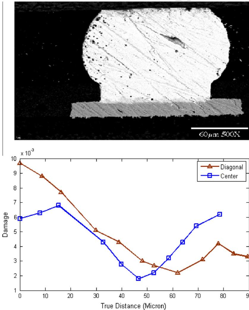
Fig. 11. Damage distribution along diagonal cross-section of the solder joint after 6.7 h 0.1 Hz PDC loading at duty factor of 0.5.
