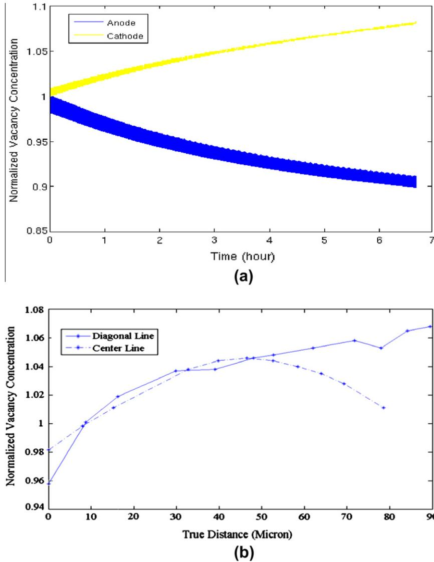
Fig. 4. Vacancy concentration evolution history under pulse current loading of 0.1 Hz and duty factor of 0.5: (a) vacancy concentration evolution at corner A and B and (b) vacancy concentration along diagonal cross-section A-B and center cross-section C-D after 6.7 h pulse current loading.
