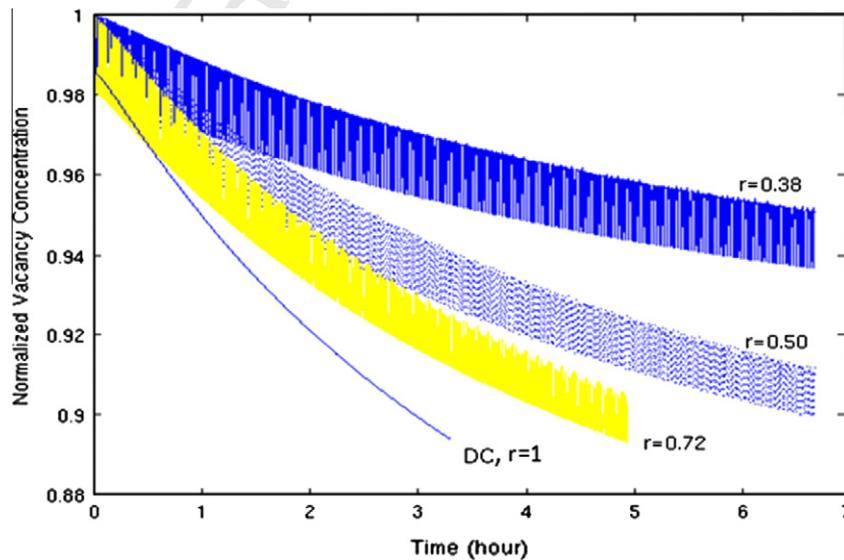
Fig. 5. Duty factor  $r$  dependence of vacancy concentration during current loading history at corner A (anode) of solder bump, with frequency of 0.05 Hz.
