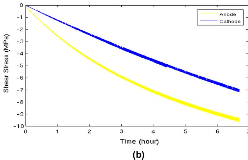
Fig. 7. Volumetric and shear stress evolution at anode and cathode of solder bump during pulse current loading history of 0.05 Hz, duty factor of 0.5: (a) volumetric stress and (b) shear stress.
