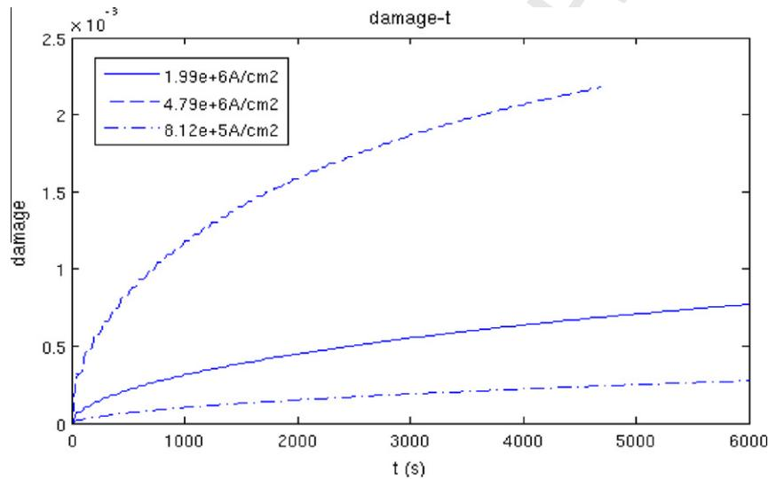
Fig. 14. Maximum current density dependence of damage evolution at cathode side of the solder joint subjected to 0.05 Hz PDC loading with duty factor of 0.5.
