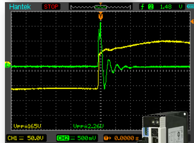
Rise edge of drive pulse (yellow trace) Green: ground current
