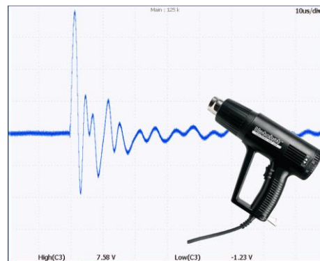
Figure 1. Power line transient from turning on heat gun.
