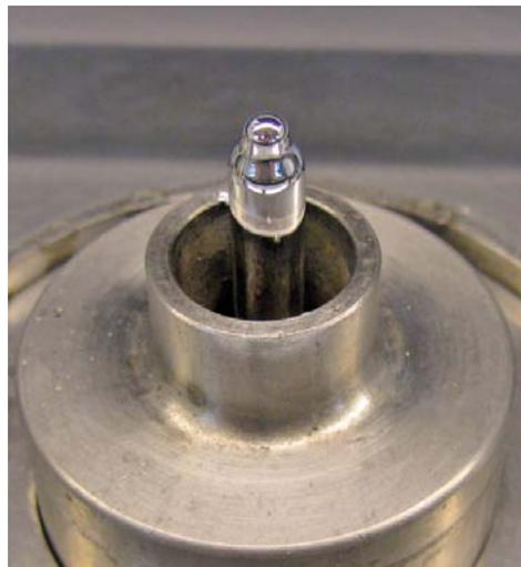
*Dross can clog small nozzles if it gets into the solder flow..*
