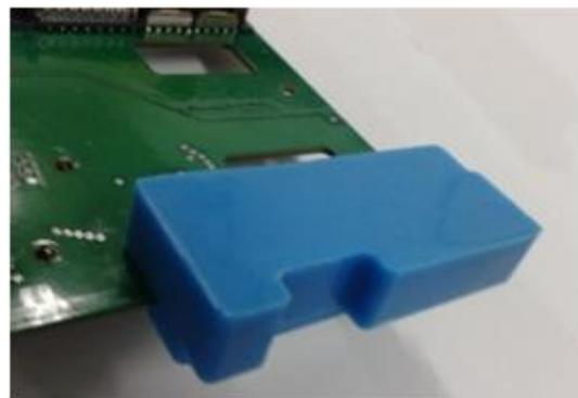
Figure 5: Masking a complex component like this is done in seconds with a boot compared to hand masking with tape.
