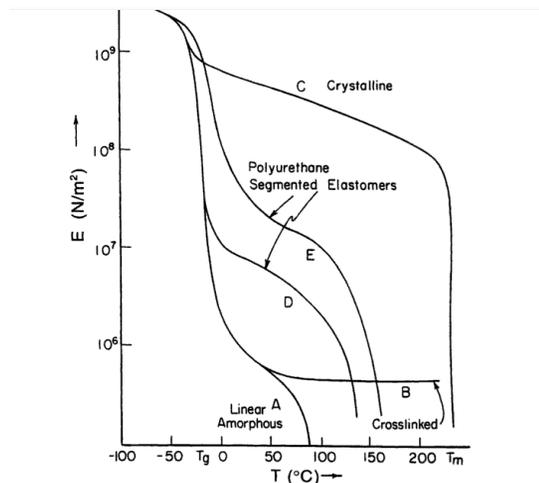
FIGURE 22 Storage modulus v temperature curves for (A) linear amorphous polymer, (B) crosslinked polymer, (C) semicrystalline polymer, (D) MDI/BD/PTMA segmented polyurethane (32% MDI by weight), (E) MDI/BD/PTMA segmented polyurethane (38% MDI by weight). From Cooper S.L. and Tobolsky A.V.J. *Appl. Polym. Sci.*, 10:1837, Copyright 1966. Reprinted with permission by John Wiley & Sons.
