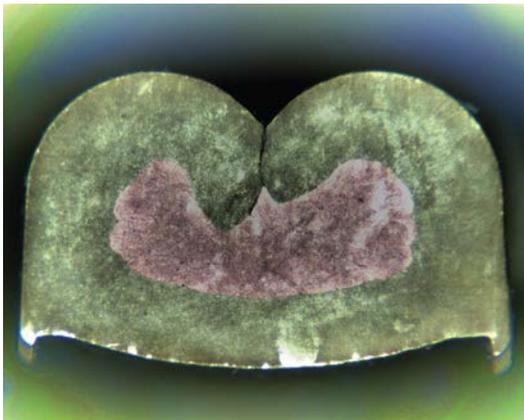
Micrograph analysis of crimped wire
