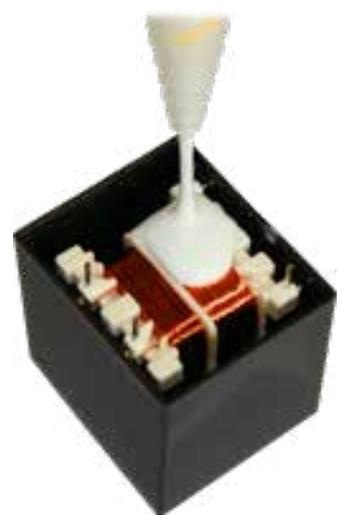
*Air bubbles during potting compromise how electronic components function in many ways – whether a component is potted in a vacuum or under ambient air conditions, what ultimately matters are the requirements for a quality component*
