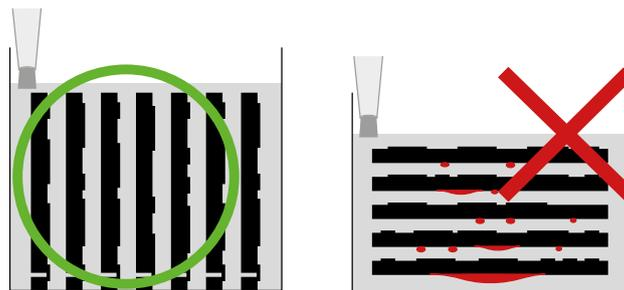
Vertical arrangement compared to horizontal arrangement of workpiece surfaces
