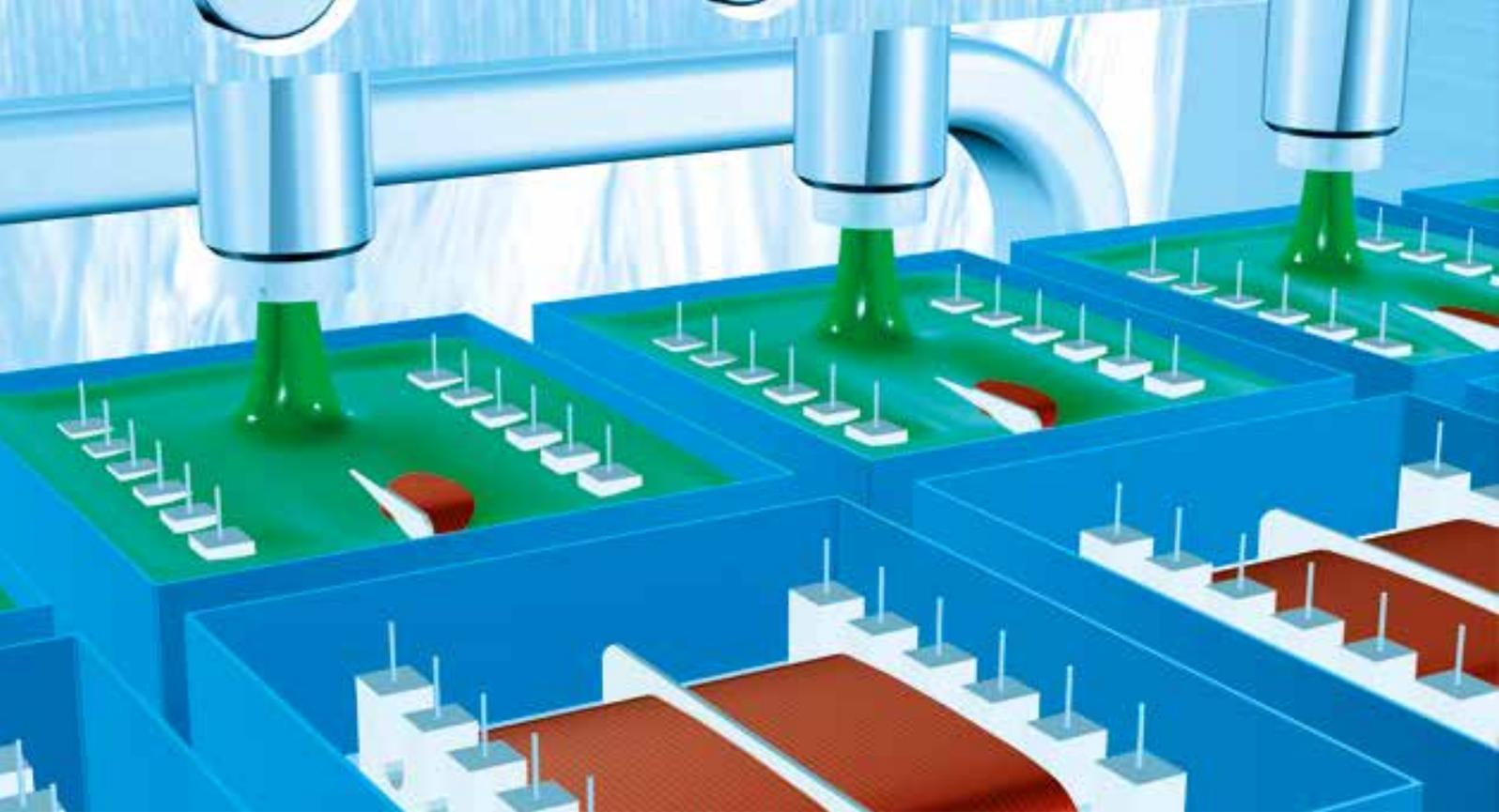
Potting solenoids with a multi-nozzle dispenser in a vacuum
