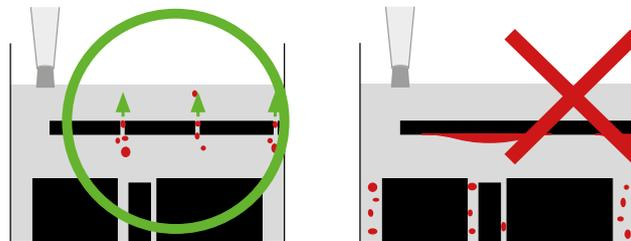
Horizontal workpiece surface with and without vent holes
