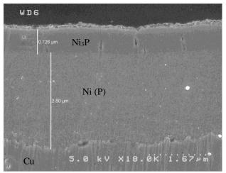
**Figure 2.** Cross-section of solder pad affected with blackpad. The  $Ni_3P$  layer is less than a micrometre thick and shows cracks.
