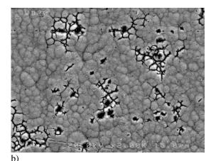
**Figure 3**. Blackpad affected board exposed to humidity. a) optical cross-section image across a blister bubble. b) Planview SEM image of another region of the same part. The mud cracks are very visible in SEM because they are coated with the ENIG gold plating layer. They are also visible in the optical cross-section, once one is acquainted with their appearance. The blue arrow in (a) points to such a crack. A few more are visible if you look carefully.
