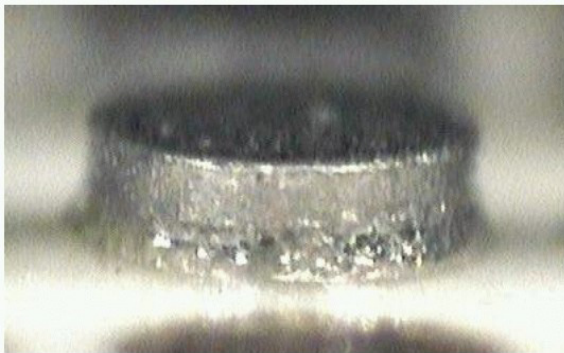
Figure 5 - Reflowed Preform Side View
