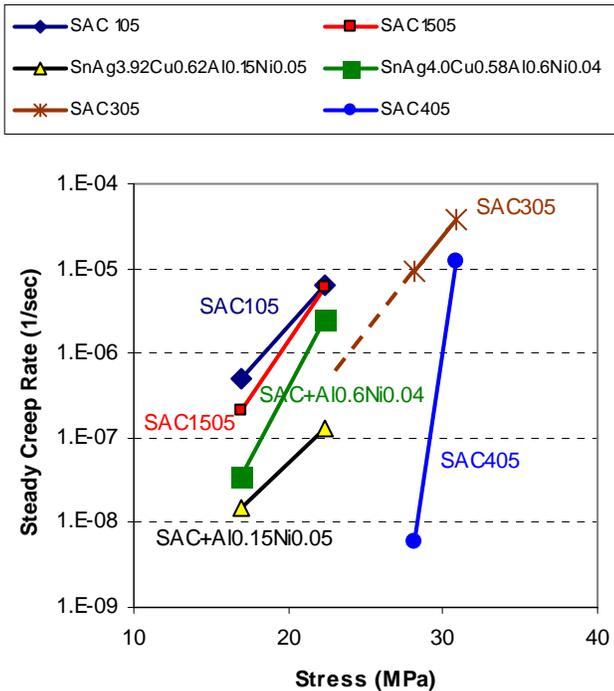
**Fig. 21** Effect of alloy on steady creep rate.
