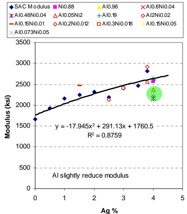
**Fig. 6** Effect of alloy composition on modulus.
