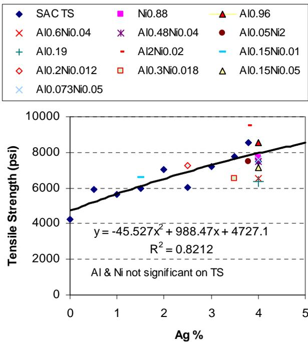
**Fig. 4** Effect of alloy composition on tensile strength
