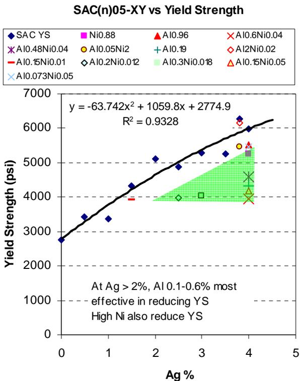
**Fig. 1** Effect of alloy composition on yield strength.
