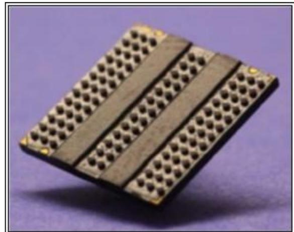
**Figure 8.** Bottom view of a completed two die DFD package assembly.
