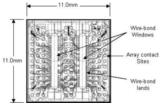
**Figure 3.** Substrate developed for the dual face-down package (bottom view).
