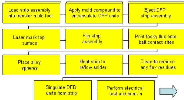
**Figure 7.** Second phase DFD package assembly process sequence.
