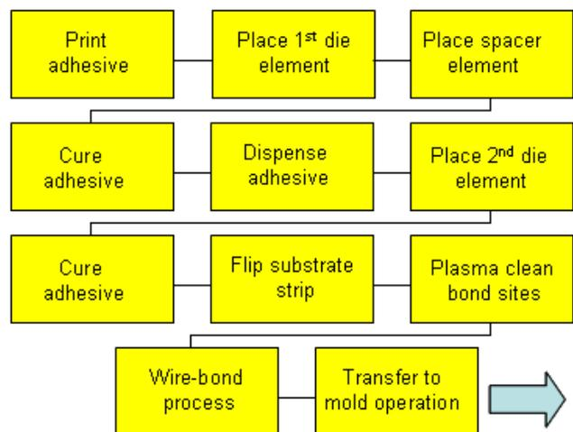
**Figure 5.** First phase DFD package assembly sequence.
