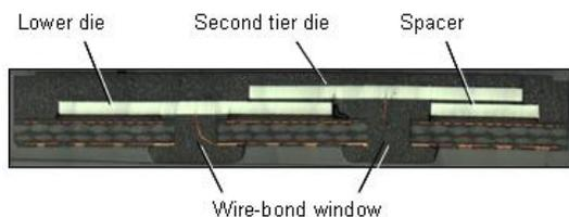
**Figure 4.** Cross section of face-down offset wire-bond.
