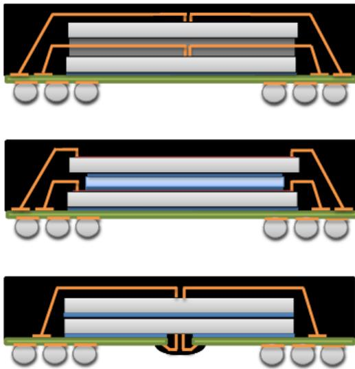
**Figure 1.** Multiple die memory package assembly variations.
