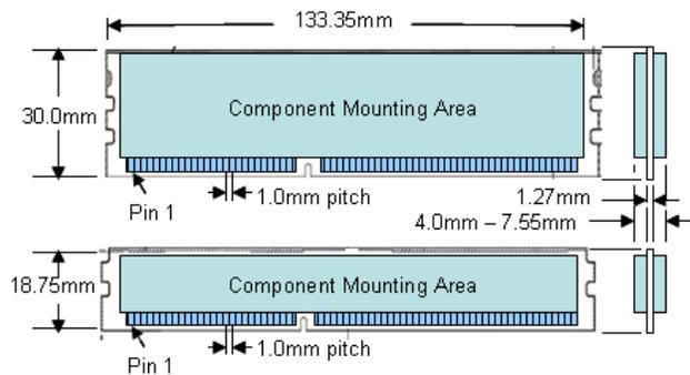
**Figure 10.** Comparing low profile and very low profile DIMM module outlines.
