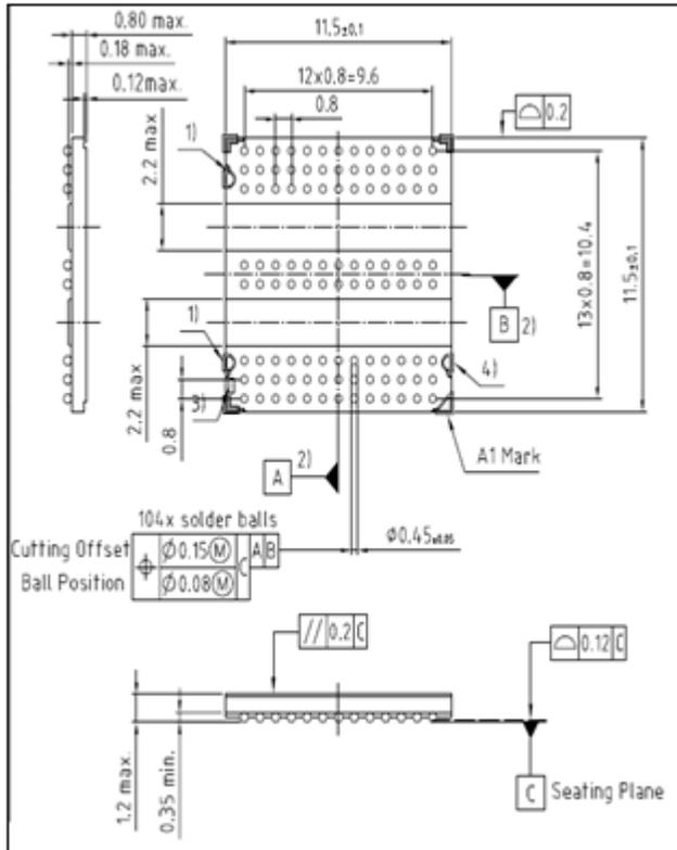
**Figure 9.** Mechanical outline detail for the Invensas two DDR3 die, face-down wire-bond package.
