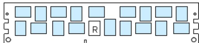
**Figure 11.** DDR memory DIMM with single die packaging.
