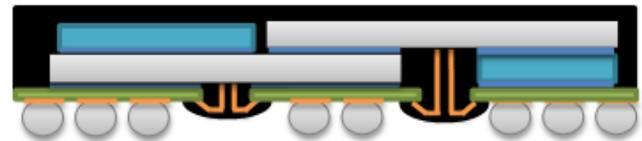
**Figure 2.** Invensas 'dual face-down package' for center-bond DDR memory.
