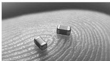
Figure 1: In 2004, Murata Manufacturing Co., Ltd. introduced the market's smallest chip component: the 01005 capacitor (0.01 x 0.005 inch; 0.4 x 0.2 mm or 0402Metric).
