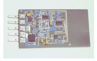
IRC produces this Anotherm® aluminum alloy substrates with a power supply integrating both signal and power onto circuit board acting as a heatsink. Components are directly soldered to the heatsink. **About the Author**: Tom Morris is an Applications Engineering Manager at T.T. Electronics IRC Advanced Film Division in Corpus Christi Texas, specializing in thick and thin film products. Tom has been with IRC since 1983 and is presently involved with development of thermally conductive substrates.
