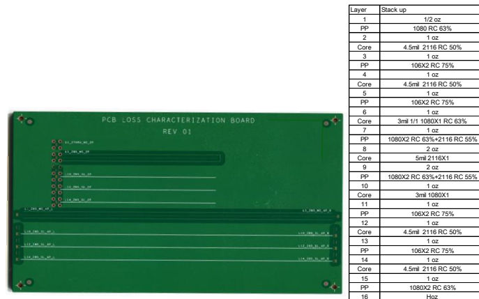
Figure 15 – Test pattern and stackup design of low loss material A
