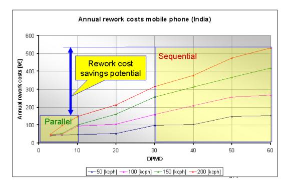
Figure 4: Rework costs DPMO and annual rework as function of line capacity.
