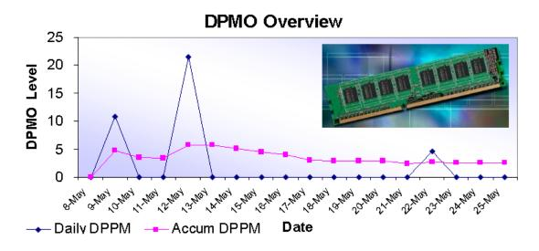
**Figure 5**: An actual line evaluation for Assembléon's AX-501 on a memory module line. Most days' production had no defects, with an average DPMO below 5.
