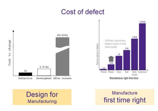
**Figure 1**: Costs of defects. At each stage the costs of correcting a defect increase by a factor 10.
