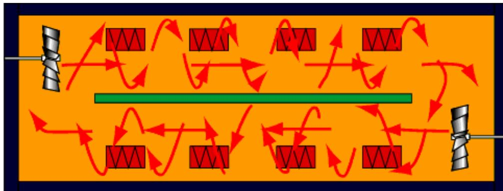
Cross-section of a GF-120HC horizontal convection oven. Air is recirculated within the confines of each chamber as shown
