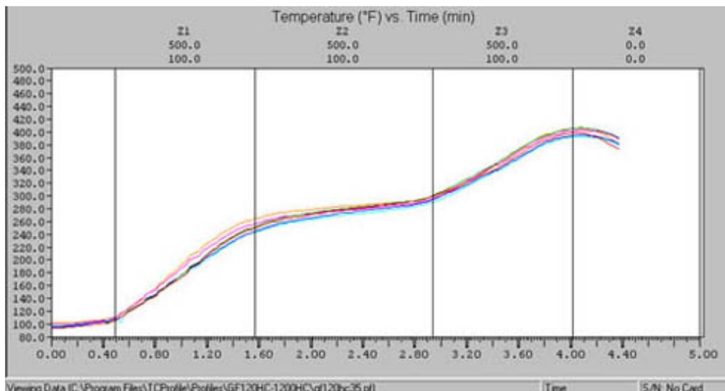
Profile taken in a GF-120HC 3 zone oven showing actual board temperatures recorded with 6 thermocouples evenly positioned across the board.
