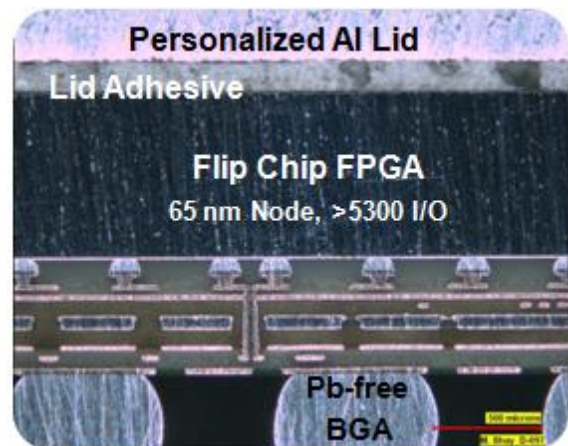
Figure 7. Cross-Section of Direct Flip Chip FPGA Attach onto HyperBGA Assembly.
