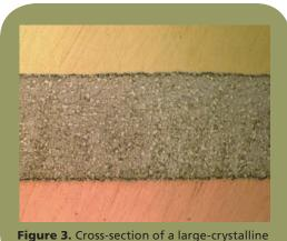
**Figure 3.** Cross-section of a large-crystalline grain structure solder joint.
