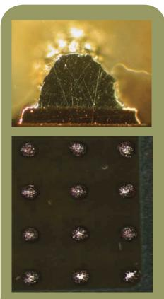
**Figure 1.** Cross-section of an acceptable solder joint with surface graping.
