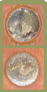
**Figure 2.** An example of good solder wetting (A) and poor wetting (B).
