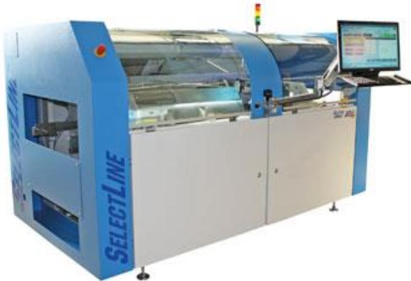
*Figure 1: Selective soldering plant (© SEHO Systems)*
