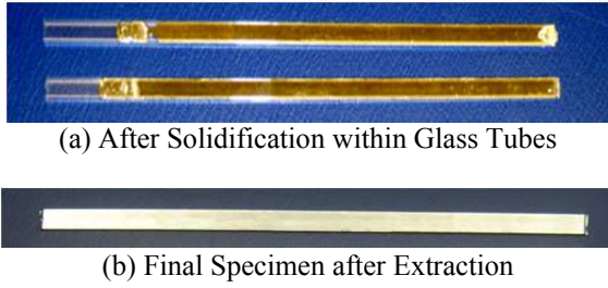
Figure 3 - Solder Uniaxial Test Specimens
