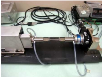
Figure 5 - Mechanical Test System with Solder Sample
