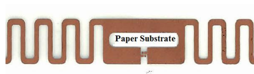
Figure 2. RFID Paper Substrate
