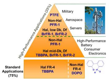
Figure 3. Flame Retardants Used in Circuit Board Markets
