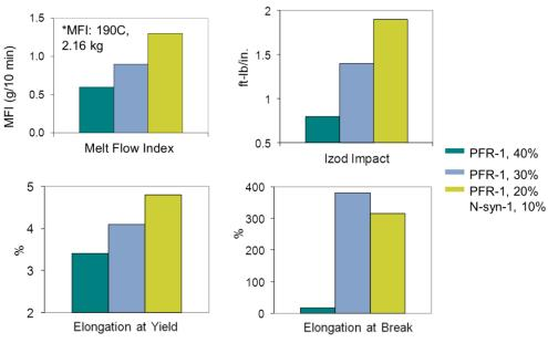
Figure 6. Physical Properties of PFR-1 in LLDPE Resin.
