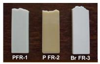
Figure 7. Flame Retardant High Temperature Polyamide Molds (3.2 mm, 1/8").
