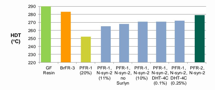
■HDT for PFR-1 with synergist (272°C) is slightly lower vs. BrFR-3 (283°C)
