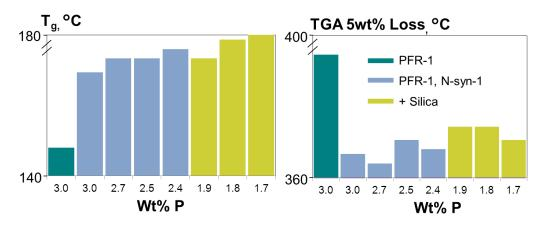
Figure 5. Glass Transition Temperature and Decomposition Temperature for Laminates Containing PFR-1.
