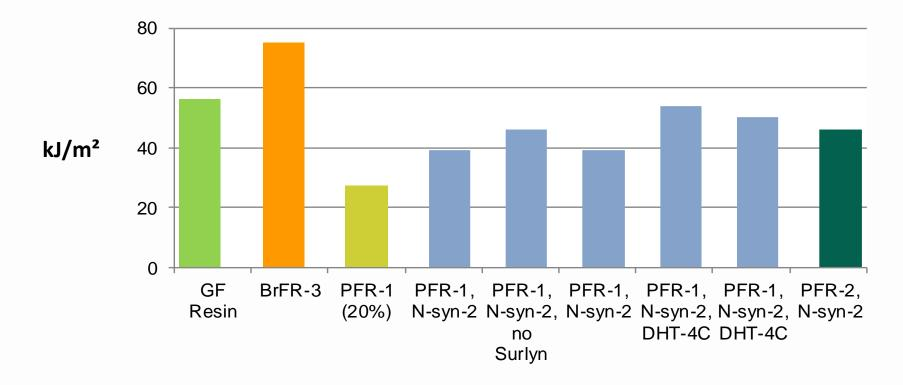
Un-notched charpy impact strength for PFR-1 with synergist (54 kJ/m<sup>2</sup>) lower vs.
