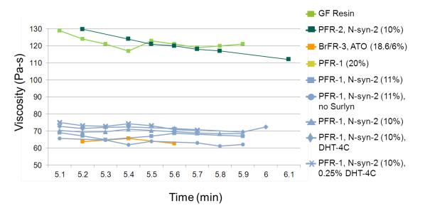
Figure 8. Capillary Rheology for Flame Retardant High Temperature Polyamide (at 1000<sup>-1</sup> sec Shear).
