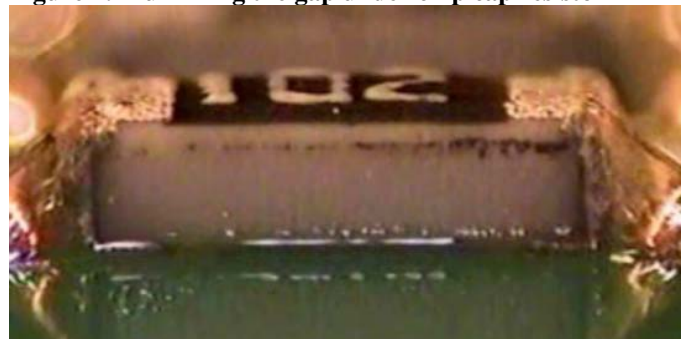
Figure 2: Flux filling the gap under chip cap resistor
