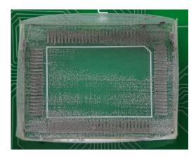
Next, the stencil can be peeled off resulting in a very consistent print volume. The stencil is designed to be discarded thereby bypassing the cleaning process and all of the problems aforementioned above.
