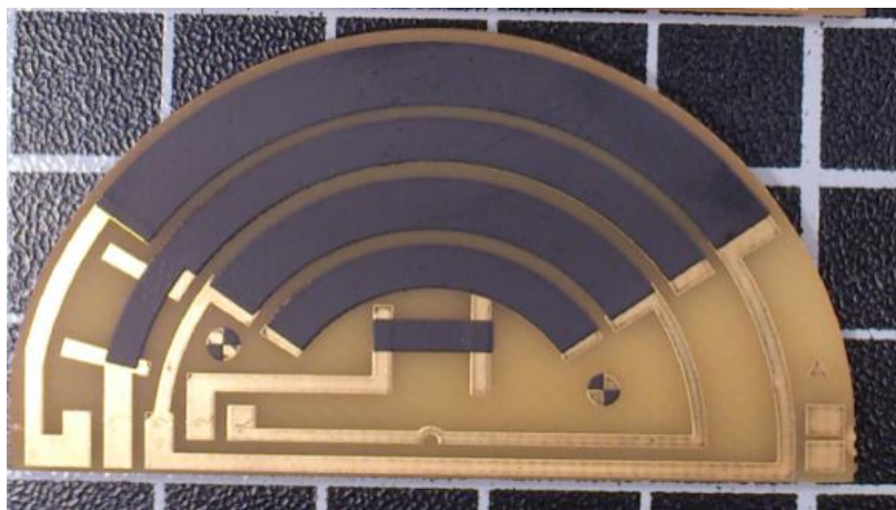
Sensor device: Printed Cu layer with metal finish
